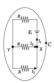
1. Write the equation for KVL for loop C.
