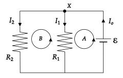
1. Use KCL at junction X and KVL for loops A and B to show that  $I_o = \mathcal{E}\left(\frac{1}{R_1} + \frac{1}{R_2}\right)$ .
