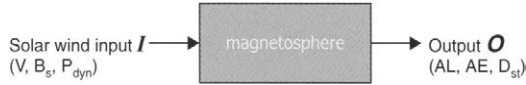
Figure 1. Representation of the magnetosphere in a data-derived approach. Input parameters are represented here by the solar wind speed v , southward component of the interplanetary magnetic field B_s , and dynamical pressure P_{dyn} , while the output is represented by the auroral indices AL and AE reflecting the substorm activity, and the disturbance storm-time index D_{st} .
